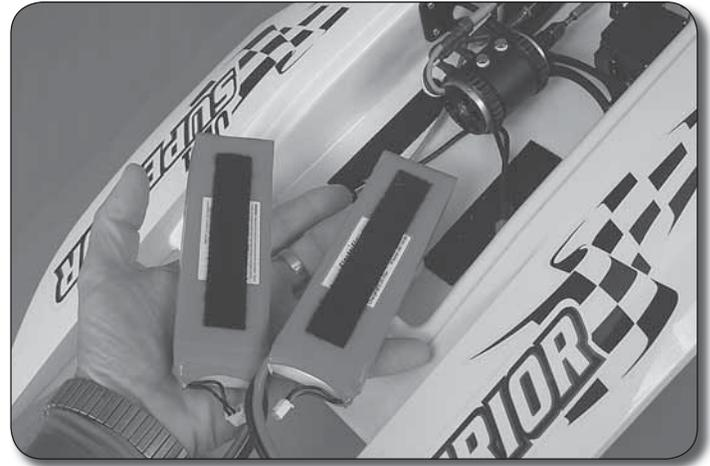
3. Install the provided hook and loop onto your LiPo batteries.
