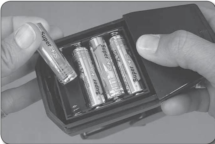
2. Install the batteries following the diagram in the bottom of the battery tray.
